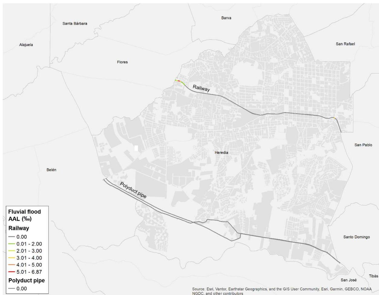
Figure 46. Average Annual Loss due to fluvial flooding for the rail and hydrocarbons sectors in the canton of Heredia
