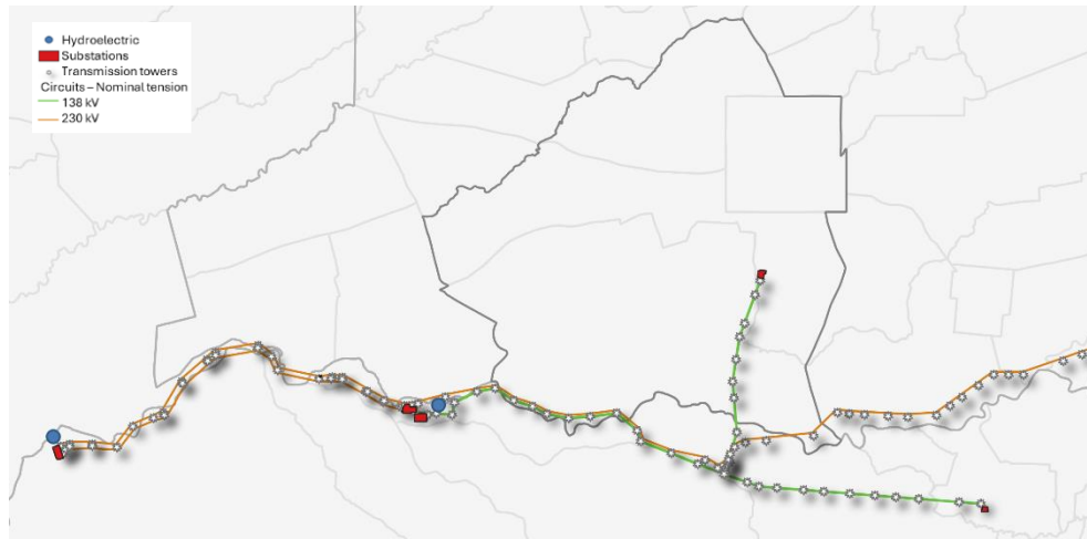
Figure 28. Power generation and transmission system for the canton of Heredia.
